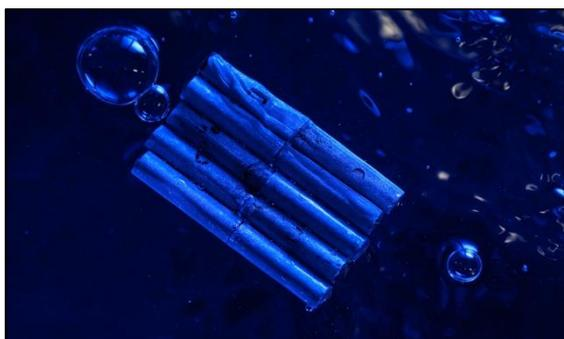
Researchers at the University of Rochester have developed aluminum tubes that remain buoyant even when submerged for long periods or heavily damaged. By engineering the metal surface to repel water, the tubes trap air inside and resist sinking. The approach could eventually support unsinkable ships, floating platforms, and wave powered energy systems.
