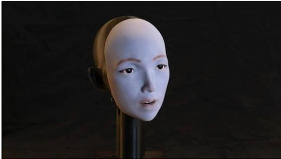
Engineers at Columbia University School of Engineering and Applied Science have developed a humanoid robot that learns realistic lip movements by observing itself and studying human videos, a step that could help robots cross the uncanny valley. Humans focus heavily on lips during conversation, and even small errors in facial motion can make robots seem unsettling. While robotics has advanced in walking and grasping, facial expression has remained a weak point.
