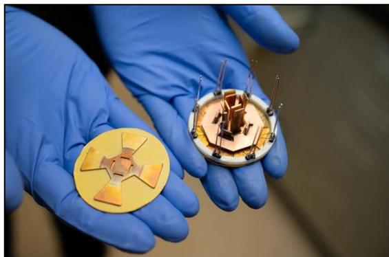
Researchers at the National Renewable Energy Laboratory have introduced a compact power module designed to make electricity use far more efficient. Called ULIS, the silicon carbide based device delivers higher power density while reducing energy losses and manufacturing costs. The innovation could help meet rising global electricity demand from data centers, manufacturing, transportation, and future energy systems.
