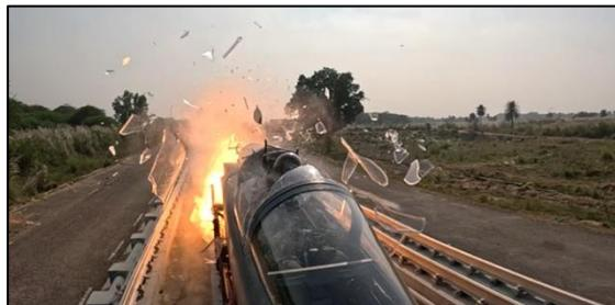
The Defence Research and Development Organisation has successfully conducted a high speed rocket sled test of an indigenously developed fighter aircraft escape system, marking a major advance in India's aviation safety and self reliance capabilities. The test was carried out at the Rail Track Rocket Sled facility of the Terminal Ballistics Research Laboratory.
